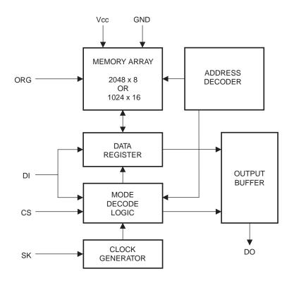
Note: When the ORG pin is connected to Vcc, the x 16 organization is selected. When it is connected to ground, the x 8 organization is selected. If the ORG pin is left unconnected and the application does not load the input beyond the capability of the internal 1 Meg ohm pullup, then the x 16 organization is selected.
