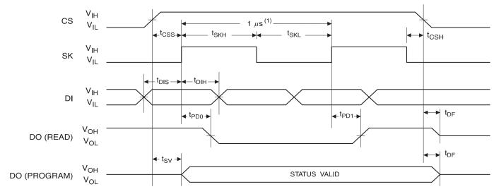
Figure 2. Synchronous Data Timing
